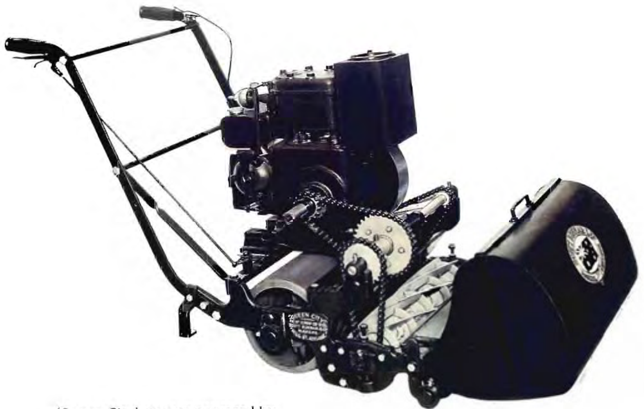
'Queen City' mower powered by a Ronaldson Tippet't'N' type motor.
