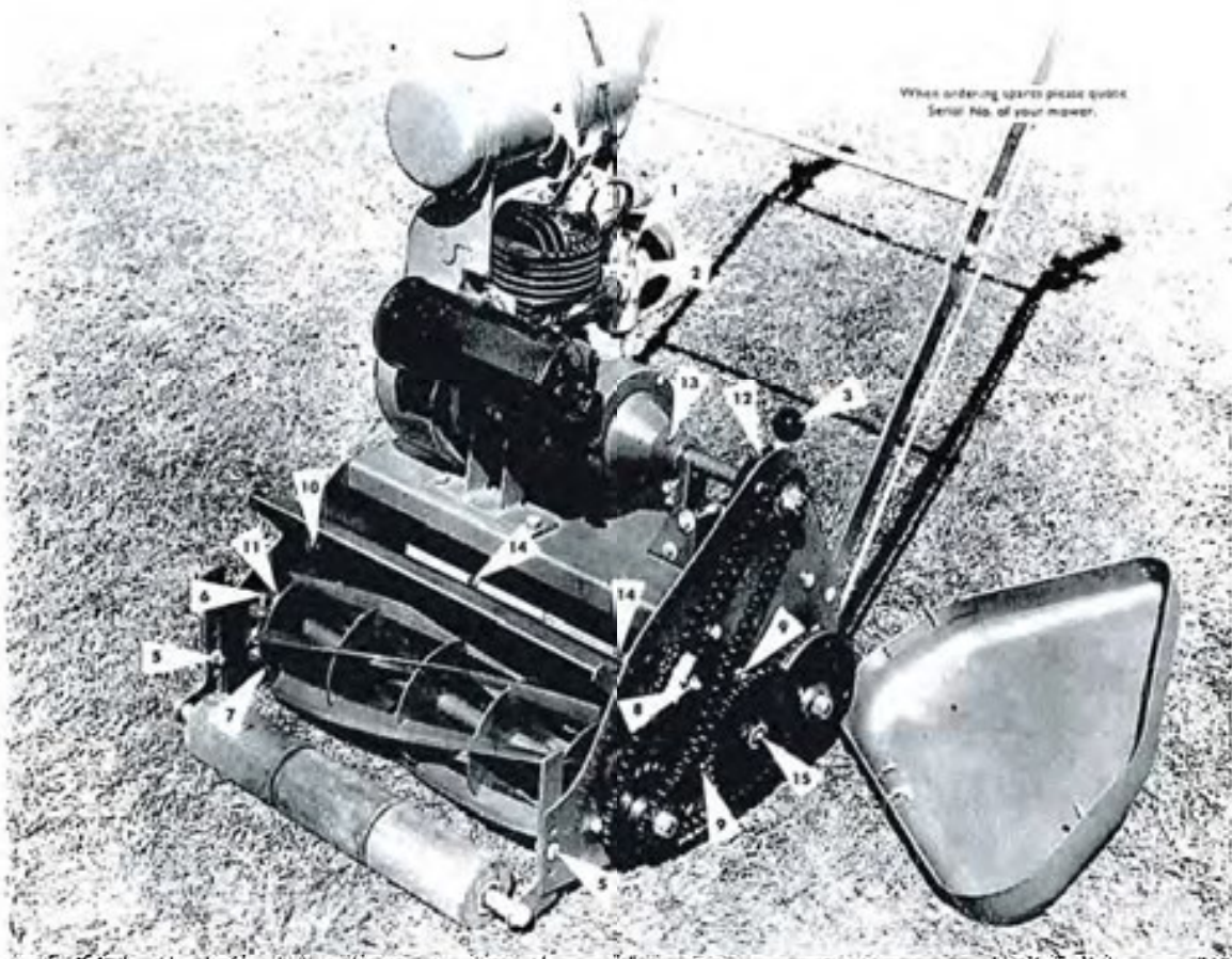
www.outdoorliving.com A Scott Bonnar 16' Model 33 mower with a Villiers 98cc Mark 3 Midget 2 stroke engine.
