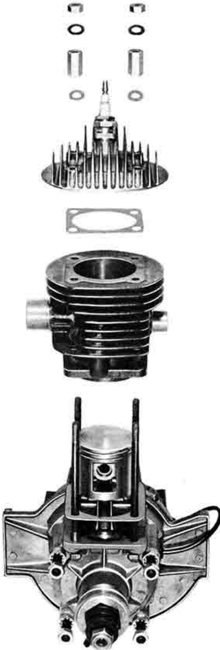
View of cylinder head and cylinder barrel removed from 160cc engine. Early models.
