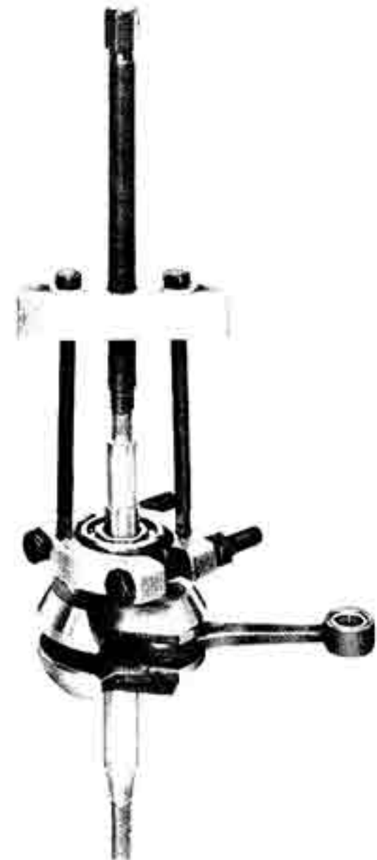
Remove the bearings from the crankshaft using a suitable puller.
